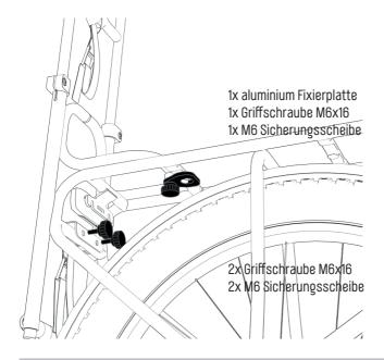
1x alloy fixing-plate 1x handlever M6x16 1x M6 lockwasher
