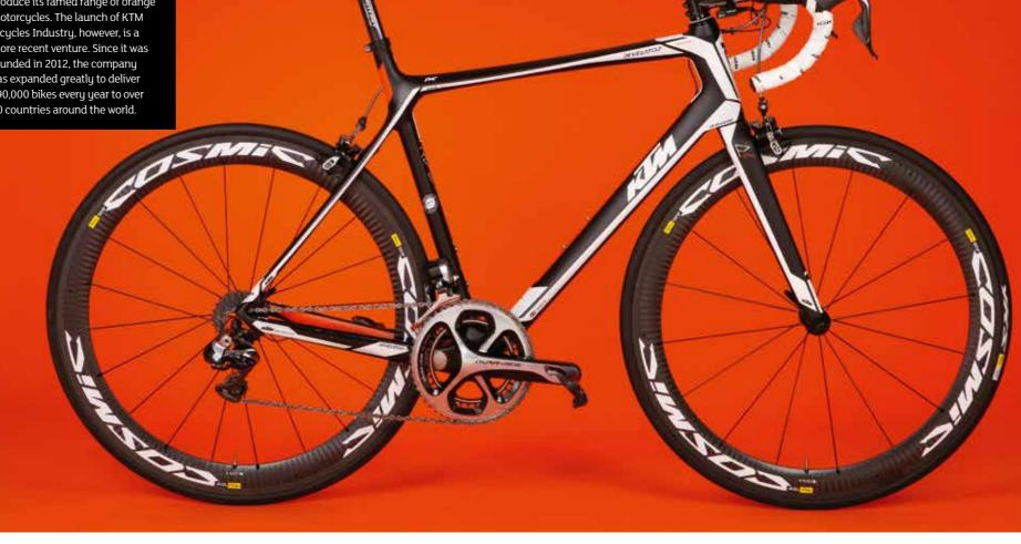
For the rider to get the most out of their efforts, whether it's in a race or smashing a PB on Strava, it's imperative that no power is lost in the frame's chassis. The Revelator Prestige is fitted with the new PressFit Shimano BB72-41B bottom bracket and paired with oversized chainstays, so the rider's efforts are immediately turned into motion.
